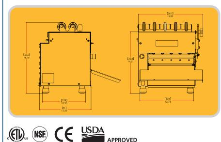
Rollers: 3.5" (9cm) dia. by 11" (28cm) length Scrapers: Synthetic, Spring Loaded, Removable Bearings: Sealed Ball Bearings, Permanently Lubricated Gear Motor: Heavy Duty 1/4 HP, Maintenance Free, Single Phase,
