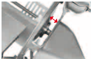
Increased gap between blade and machine body
