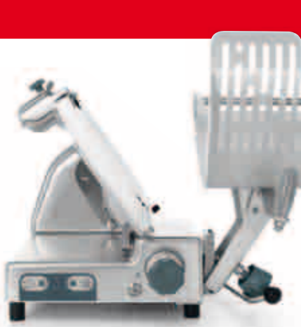
Tilt-carriage with zero blade exposure
