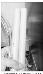
Chemical Pick-up Tubes. stiffener tubes & line strainers.
