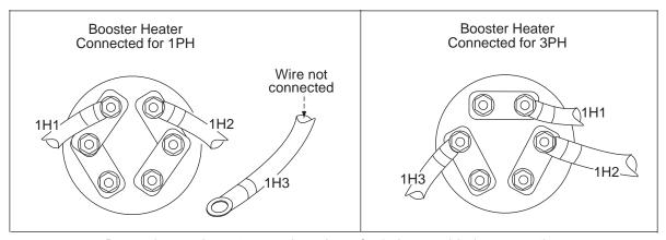
Booster heater element connections shown for 1 phase and 3 phase operation.
