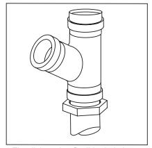
The dishwasher flexible drain hose must be connected to a WYE fitting.
