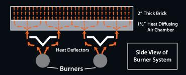
As the special air chamber located below the cooking surface eliminates hot spots and eliminates the need to rotate pies, an exclusive baffle system using slots instead of circles push more heat to the center of the oven, cooking your pies evenly on top and providing for a crispier, evenly baked pizza.
