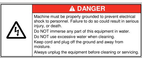
Your electrician must furnish sufficient power for proper machine operation. We recommend this shaver be on a dedicated and protected circuit. Failure to wire properly will void the warranty and may result in damage to the machine. It is Gold Medal Products Company's recommendation that this machine be plugged directly into a wall outlet. The use of extension cords is not recommended due to safety concerns, and may cause sacrificed and/or reduced performance.
