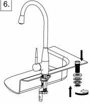
From the top of the installation hole, the bottom of the hole, install the decorative cover (11), washer (12), metal washer (13), and locknut (14).
