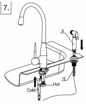
Install the water supply pipes to the main body and the spray hose (16) to the side spray (9) and check valves.
