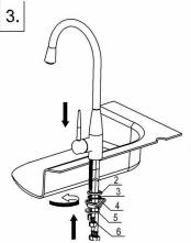
Place the main body onto the sink and adjust it to the desired position. Install the down ring (2), rubber washer (3), plastic washer (4), metal washer (5) and locknut (6), using the S14 sleeve wrench to tighten.
