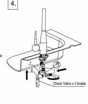
Install the washer (7) and diverter (8) to the main body, using the wrench to tighten the diverter. Wrap PTEE tape to the thread of the diverter and install the G3/8 inlet pipes to the main body.
