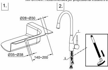
Make two holes: faucet hole diameter Ø35~Ø38mm, side spray hole diameter S14 sleeve wrench (15) to screw out Ø28~Ø30mm. The distance between two holes: 140~200mm.
