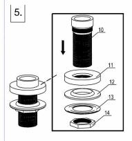
Take out the side spray assembly. Remove the locknut (14), metal washer install the side spray seat (10). From (13), washer (12) and decorative cover (11) from the side spray seat (10).
