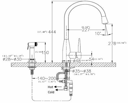
1. Leave enough distance between the installation hole and the wall to make sure the faucet handle can be fully pushed backward (minimum distance: 3.5").
