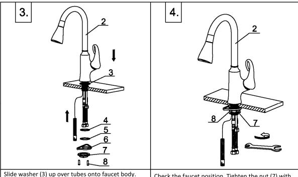
Slide washer (3) up over tubes onto faucet body. Place tubes through mounting hole and slide faucet down until it rests on mounting surface. Slide 8, 7, 6, 5 and 4 up over tubes onto faucet body.
