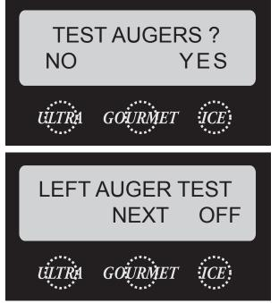
Select NEXT to repeat process for Right Auger Test. NOTE: ULTRA-1 models will only have one test screen.
