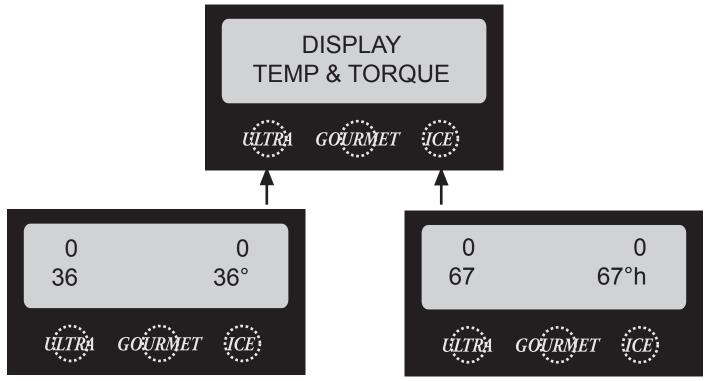
**NOTE:** ULTRA-1 models will display Barrel Temperature and Torque readings on the left side of the display.
