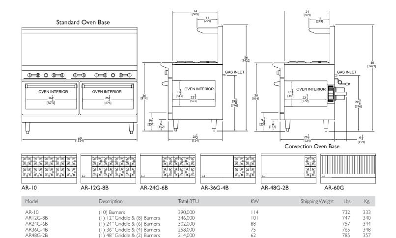
Optional Innovection base available: Add Suffix '-NV'. 'NVL' for oven on left side or 'NRV' for oven on right side. Optional Convection base available: Add Suffix '-C'.'CL' for oven on the left side or 'CR' for oven on right side.
